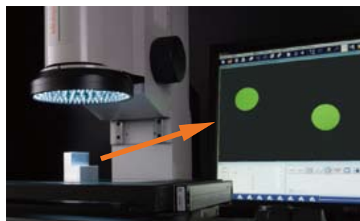
Focusing in on a workpiece like the one shown above is unnecessary.
